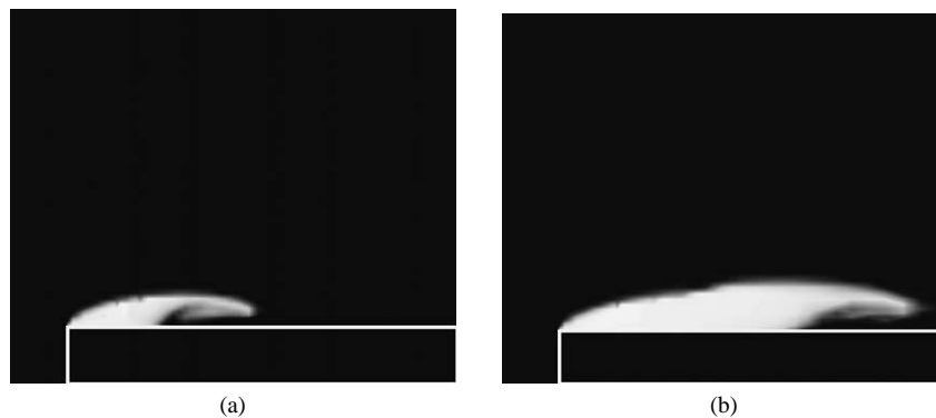
Fig. 9. Bubble shape of the cavitating flow over an axisymmetric blunt body: (a) \sigma = 0.5 , (b) \sigma = 0.3 .
